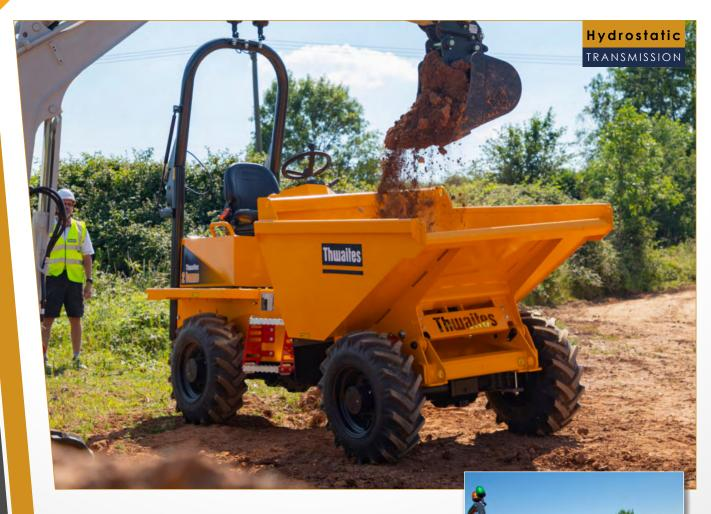
The Thwaites 2 Tonne Front Tip, Stage V dumper is manufactured with contractors and hirers in mind – ensuring operator safety, reducing risk on site and improving performance. Powered by an 18.1 kW 3-cylinder Yanmar engine, delivering 107 Nm max torque for optimum traction and control. The Thwaites 2 Tonne Front Tip is also available with a Manual Transmission.
